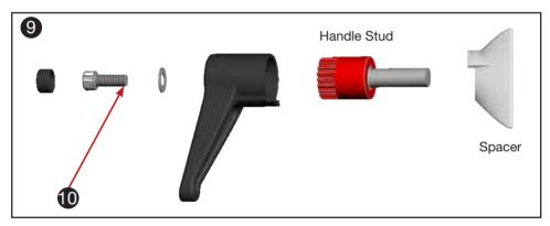
Step 11: Assemble Handle Stud and the Handlebar Spacer.
