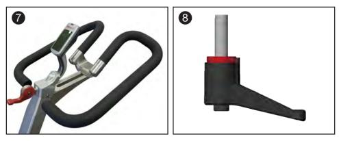
Step 9: Using a 5mm Allen wench remove the Screw and Washer, releasing the Handle Stud.Step 10: Clean Screw thread with alcohol, then apply Loctite 242 to leading edge of screw thread for handle bar adjust screw.
