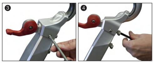
**Step 3**: Using a 6mm Allen wrench, and the four screws, assemble the Bottom Slide to the Handlebar Tube. Tighten firmly, making sure there is no gap between the Slide and the Handlebar Tube (Fig. 6).
