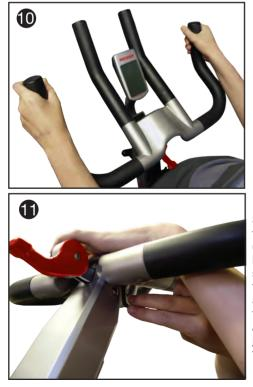
**Step 1:** Obtain the handlebar assembly, 6mm Allen wrench, and the socket head cap screws (M8x1.25 X 12 SS). Observe the location of the two mounting flanges on the handlebar post. Place the handlebar assembly on the post mounts, aligning the mounting holes. (Fig. 10).
